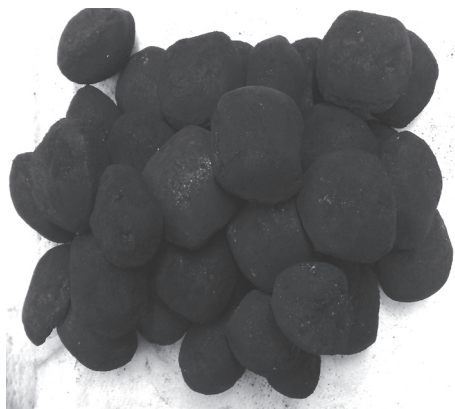
The recommended maximum multi fuel load: Photo shows a typical fuel load of approximately 1.5kg of approved smokeless ovals
