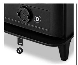
Use the tool provided to adjust the Secondary air control A – moving it to the left hand side will reduce the air supply and 'slow' the fire down. B is Primary air – move clockwise to close
