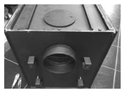
The flue and blanking plate are then swapped over. Be careful to ensure good air-tight seals are maintained on the new attachments – use fire cement if necessary
