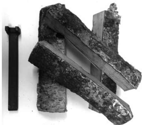
The recommended maximum fuel load: Photo shows a typical loosely stacked fuel load of approximately 1.5kg of fully seasoned wood logs approx 250mm (9") long by 75 – 100mm thick
